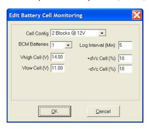
Clicking the 'Bat Mon' Edit Button in the SCU screen will cause the screen show to the left to appear. This screen allows configuration of the optional Sageon® Battery Monitor.
