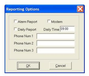
Clicking the 'Reporting Options' Edit Button in the SCU screen will cause the screen show to the left to appear. This screen allows configuration of the remote reporting feature available for Sageon® Power Systems equipped with the modem interface.
