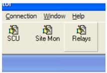
Allows the display and editing of the Relay Configuration Parameters. The same can be achieved by selecting Relays -Display Parameters.
