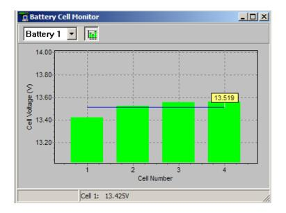
Histogram display of battery cell voltages.
