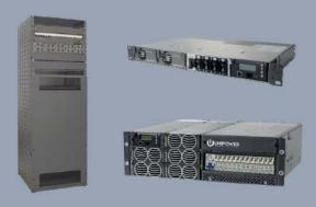
Aspiro family are 1RU and 2RU rack-mount systems rated from 45A to 90A at -48V. All systems incorporate MCB load distribution while GMT fuse options are available. Guardian family are available as 2RU to 10RU rack-mount or floor standing cabinet based systems rated from 200A up to 3300A at -48V.
