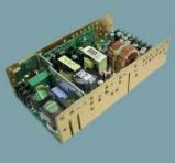
The DCMOD family offers identical features and capabilities as the EASYMOD. Most types are available with a DC input of 12V, 24V or 48V
