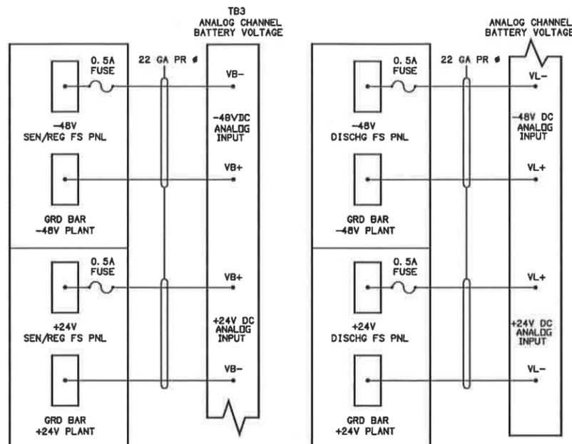
FIG 6 TYPICAL WIRING FOR HIGH VOLTAGE SHUT DOWN AND RESTART.
