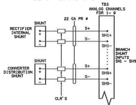
FIG 5 DISTRIBUTION LOAD MONITORING WITH SHUNT
