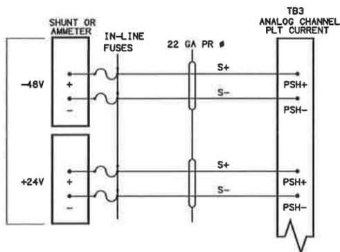
FIG 4 RECTIFIER OR CONVERTER LOAD MONITORING
