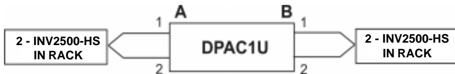
(b) INV2500-HSs in Rack (115VAC only) Connected to DPAC1U
