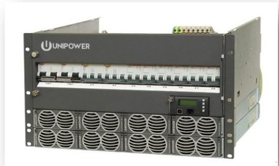
*The easy-to-install Guardian Access MS31 units are 5RU or 6RU high 19" rack-mounted, integrated DC power systems providing an output of -48VDC. These systems feature remote monitoring & control and can accommodate highly configurable systems incorporating 2 rectifier shelves with up to 8 Guardian high-efficiency hot-swap rectifiers.*
