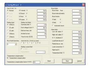
PowCom<sup>TM</sup> provides easy user access to set points for battery functions such as test, equalize, compensation, and alarm limits.
