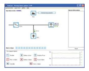
Critical system parameters, such as rectifier and alarm status, are concisely displayed.
