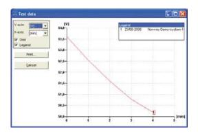
Graphical presentation of battery test data facilitates comparison with future test results for battery integrity trend analysis.
