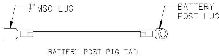
Fig. 1 Lead termination at battery cell.
